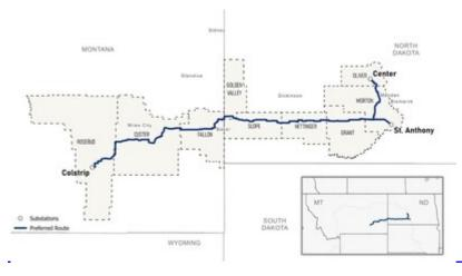
The North Plains Connector will be the nation's first HVDC transmission connection among three regional U.S. electric energy markets the Midcontinent Independent System Operator, the Western Interconnection and the Southwest Power Pool - providing additional flexibility and the sharing of resources across multiple time zones.
